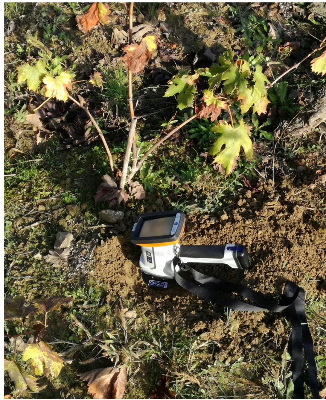
Photo 2 - In situ chemical analyses with FP EDXRF
